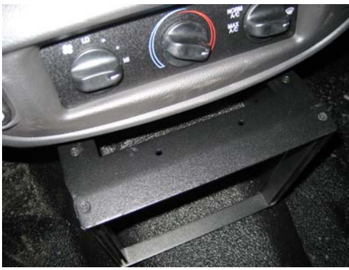
Holes are for screws to attach to the OEM dash
